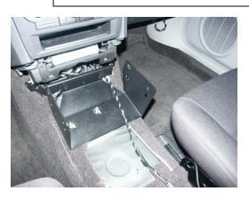
View of installation to this point Note: Be sure OEM wiring is not being crushed by mounting brackets
